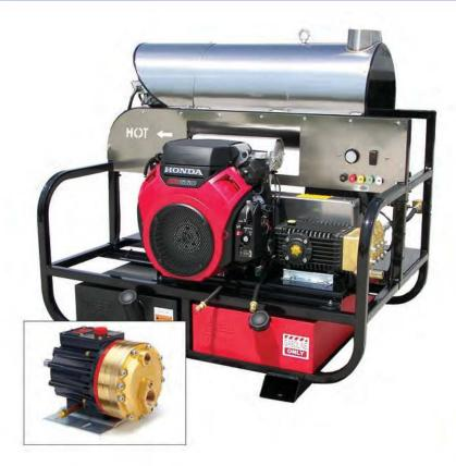
System is comprised of a portable, self contained, skid mounted hot water tank wash system, capable of driving a hydraulically operated spinner at high temperatures (195°F), 20 gpm, pressure up to 800 psi.
